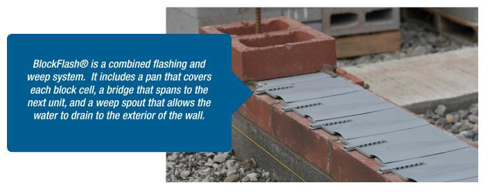
These units are available to fit 8, 10, or 12" deep CMU sizes. In addition to the pan and weep piece, we also use a mesh piece that protects the flashing and weeps from being plugged by mortar droppings during construction.
